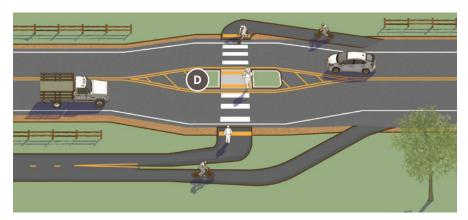
Figure 4-12. Transition from a sidepath on one side to shoulders on each side of the road.
