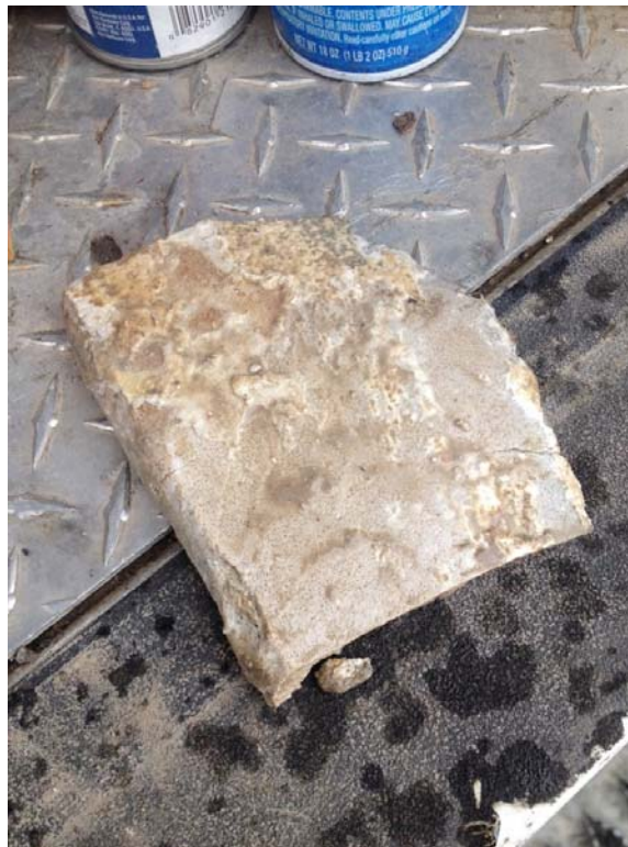
Photograph 6: View of mortar/grout from clear well interior pipe seam.
